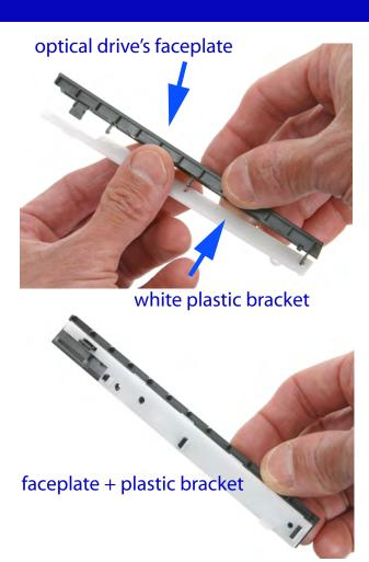
Using a screw driver gently secure the optical drive faceplate and white plastic bracket with the screw as shown (Faceplate screw).
