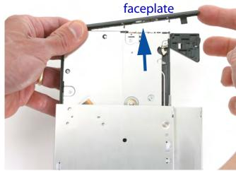
Optical drive face plate removed. It is now ready for installation on OBHD caddy
