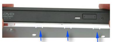
align tabs on metal caddy with notches
