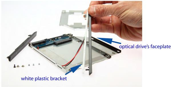
Attach optical drive's faceplate to white plastic bracket by aligning the clips on the faceplate with the holes on the white plastic bracket
